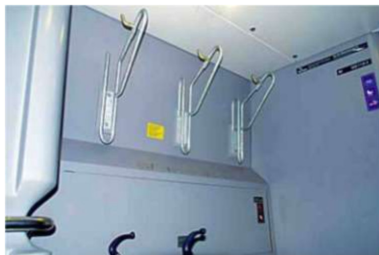
Picture 6: Storage space for pushchairs and cycles. InterCity train in Switzerland. Picture: M.Koucky
